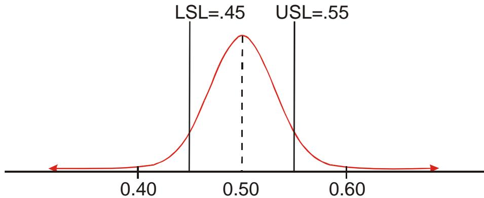
**Figure III-C 1: Example Process with  $Pp = Ppk = 0.50$**
