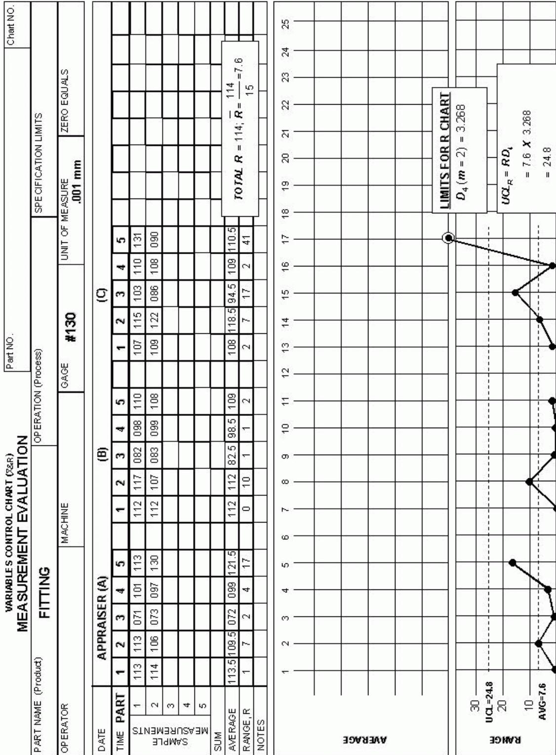
Figure IV-E 1: Measurement Evaluation Control Chart ( $\bar{X}$  & R) - 1
