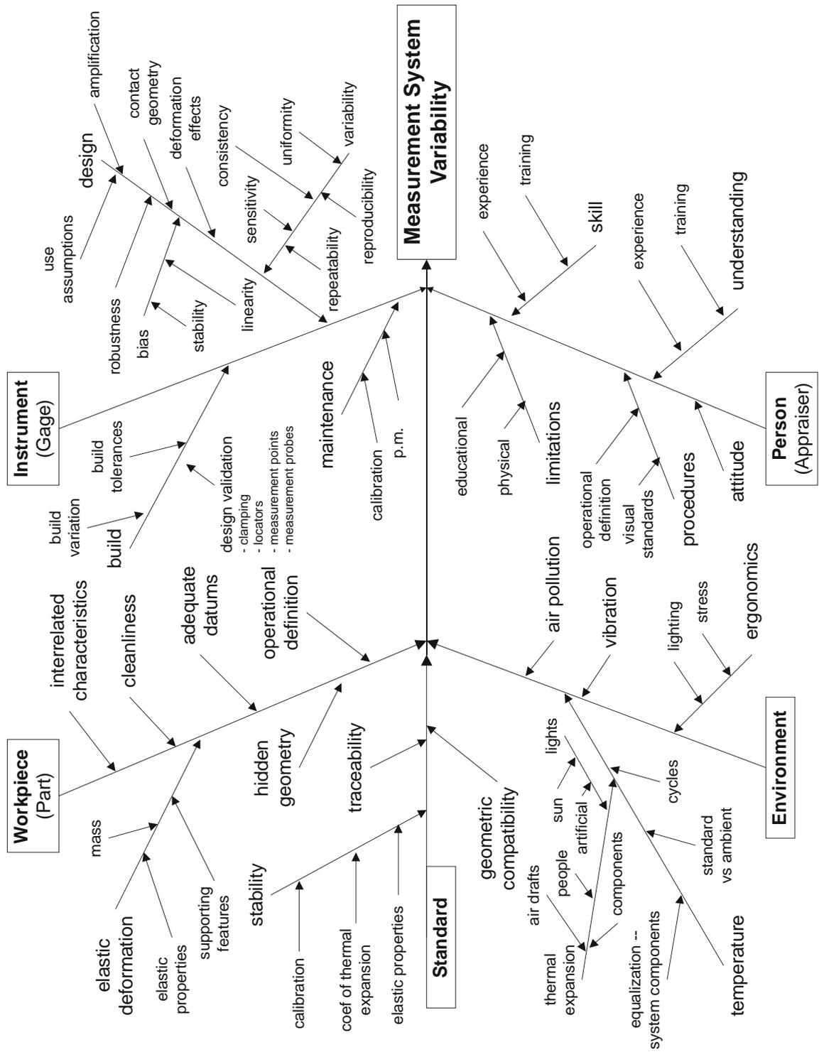
Figure I-B 1: Measurement System Variability Cause and Effect Diagram
